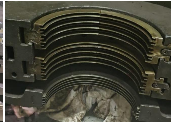
LABYRINTH PACKING (8 SEGMENTS), STEAM GUARD (1 PAIR) & OIL GUARD (1 PAIR) AFTER CLEANING
